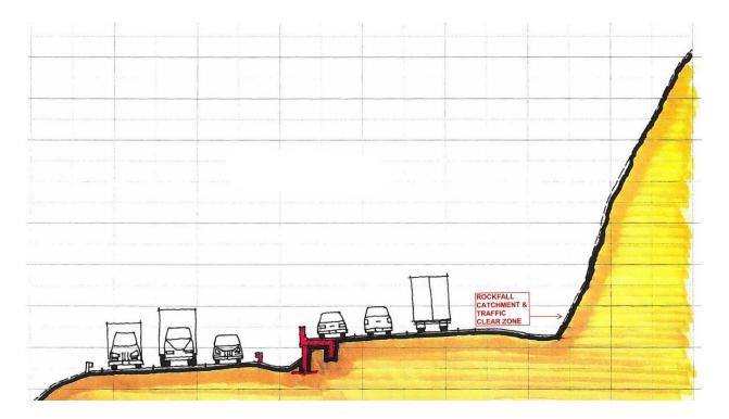
The above graphic depicts an option where the road moves toward the median and the right hand (shoulder) white line stays where it is. This prevents all lanes from getting closer to the rockfall areas. This would involve a retaining wall up to 5 feet tall near the center of the median.
